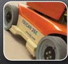
**Work Cleaner**Thick rubber non-marking tires leave facility floors intact.
